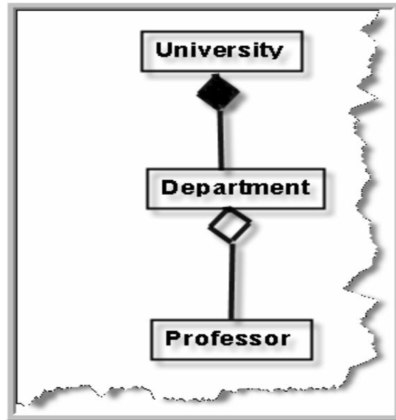
Figure 1.16: - Aggregation and composition in action
